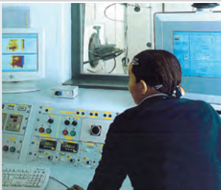
Noise is measured in an acoustic chamber
